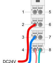
For wires with a core cross-section of 0.08mm<sup>2</sup> up to 1.5mm<sup>2</sup>.
