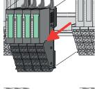
7. To mount the module group put it to the gap between the both modules and push it, guided by the stripes at both sides, to the mounting rail.
