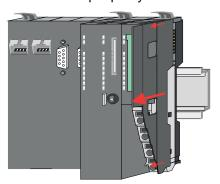
**1.** Before mounting the periphery modules you have to remove the bus cover at the right side of the CPU by pulling it forward. Keep the cover for later mounting.
