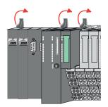
**4.** Turn all the locking lever of the CPU to be exchanged upwards.
