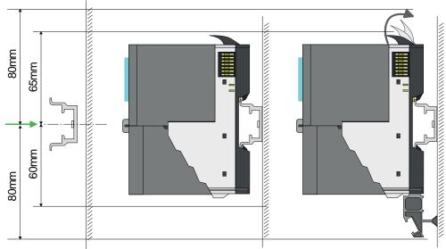
Mount the mounting rail! Please consider that a clearance from the middle of the mounting rail of at least 80mm above and 60mm below, respectively 80mm by deployment of shield bus carriers, exist.
