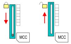
To remove, slide the sliding mechanism up again and push the storage media against the spring pressure until it is unlocked with a click.
