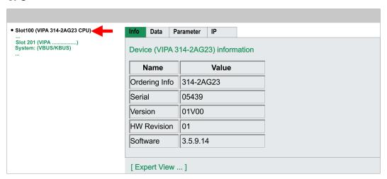
Here order number, serial number and the version of firmware and hardware of the CPU are listed. [Expert View] takes you to the advanced "Expert View".
