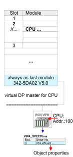
The embedding of the CPU 314-2AG23 happens by means of a virtual PROFIBUS master system with the following approach:
