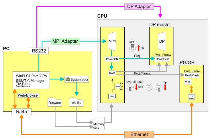
Please always use the **CPU 317-2DP (6EST 317-2AK14-0AB0 V3.3)** from Siemens of the hardware catalog to configure this CPU from Yaskawa. For the project engineering, a thorough knowledge of the Siemens SIMATIC Manager and the hardware configurator from Siemens is required!
