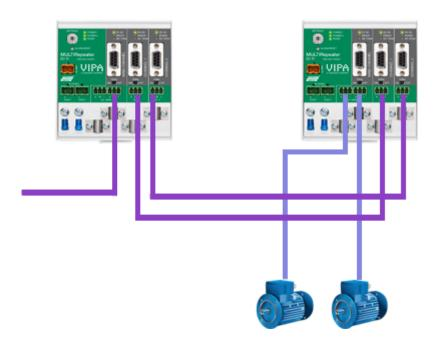
The telegrams are transferred onto both redundant channels. The logic inside the Repeater determines which telegram is used to be transferred onto the other channels. A message received by a redundant channel is repeated on all other channels, except the other redundant channel. A message received by a normal channel is repeated on all other channels.
