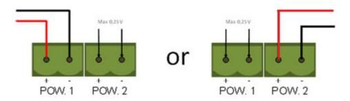
If only one power supply is used, the alarm contact is closed. If two power sources are connected, the contact is open. As soon as one of the power supplies fails, the contact will close and the Power Indicator LED will blink.
