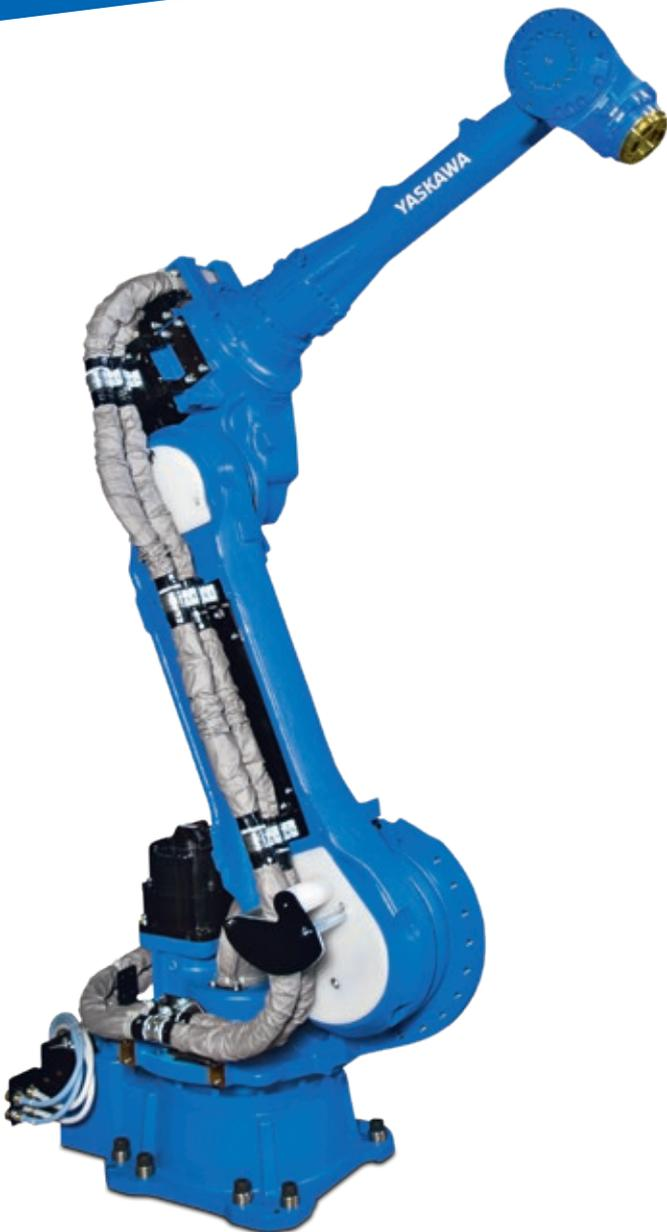
The MOTOMAN SP80 is a compact spot welding robot with 80 kg payload for servo-controlled lightweight welding guns. This technology allows very compact, cycle-time-optimized, energy-efficient and cost-effective welding cells to be installed in the smallest possible space. This robot is suitable for compact spot welding lines in car body construction with high robot density, for economical welding of small subassemblies, and for space-saving installation on a positioner.
