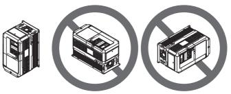
Figure 5 Correct Installation Orientation
