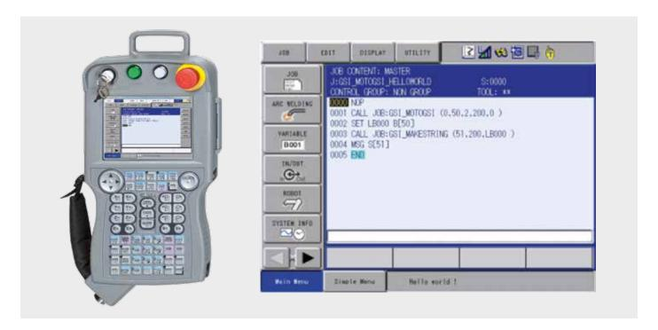
MotoGSI is a development package for creating communication interfaces on job basis. It comes with a set of jobs which allow communication with nearly every external device that supports Ethernet/TCP, Ethernet/UDP or RS232connections. It also provides a set of helper functions to process and convert the in- and outgoing datastreams which are based on byte arrays. Also included in the package is a set of sample jobs to demonstrate the way of programming.
