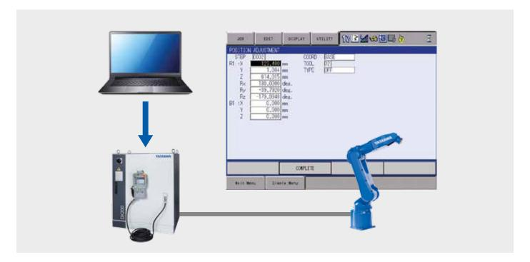
The "teaching point adjustment function" modifies the taught position data by entering the numeric number on the programming pendant without operating the manipulator.
