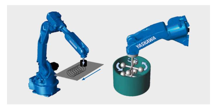
This function continuously rotates the T-axis a plural number of turns. Although the rotation angle of the T-axis is generally limited within ±360 degrees, this function allows it to rotate endlessly. When executing the move instruction MOVJ with the "number of rotations of the external axis" specified, the T-axis rotates the "specified rotating amount + teaching position pulses" during the movement to the target position. One move command can specify up to ±100 turns.
