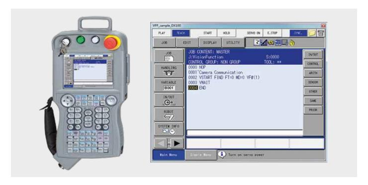
This function is an inform instruction to communicate with different Vision System. It maps the communication protocols of a variety of selected vision systems and works, dependent on these, on the basis of Ethernet or RS232. This robot instruction allows easy control of image processing devices.
